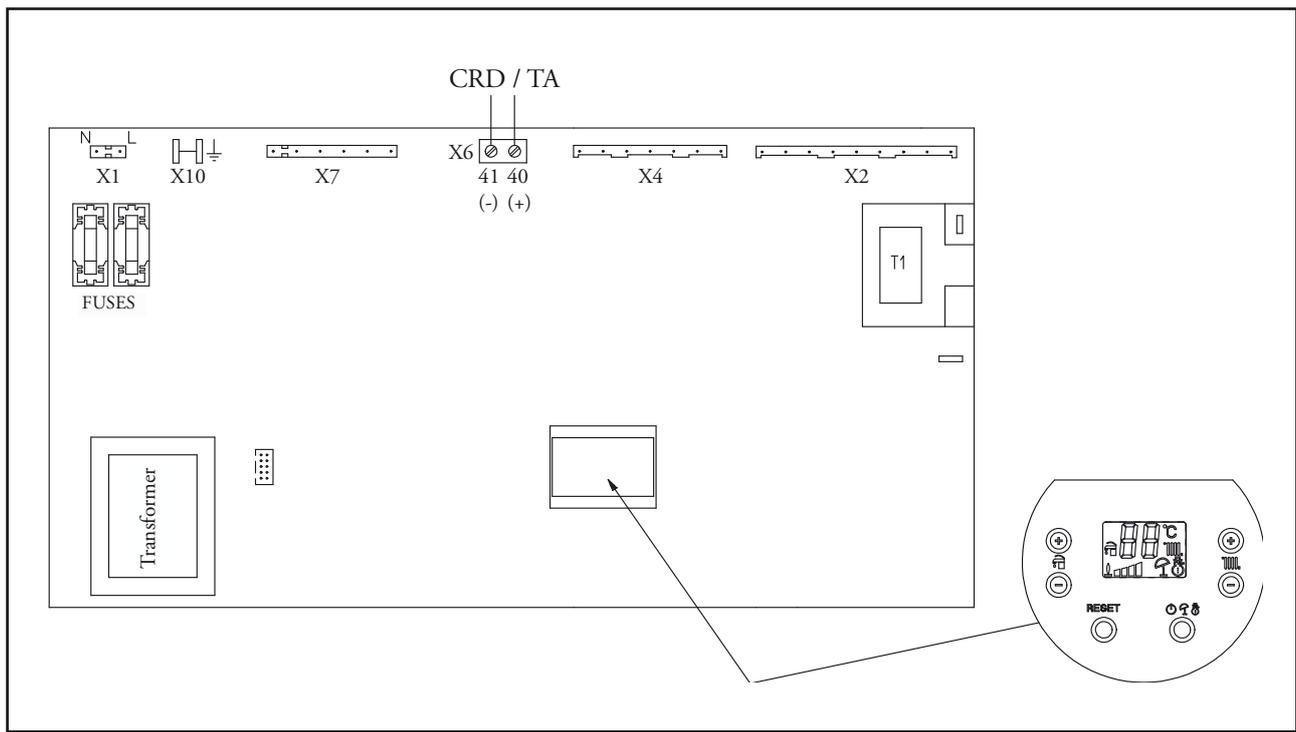
Inside the control panel the boiler is equipped with a P.C.B. with microprocessor for control of the appliance's electric devices, which takes care of linear modulation of burner power. A display shows the functioning status of the appliance, indicating any intervention of the safety devices, with which it is supplied.
