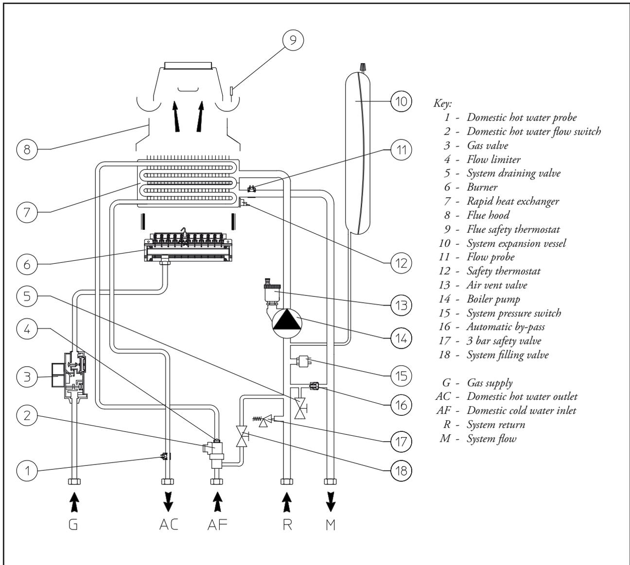
The hot water used for central heating and domestic hot water is produced thanks to two distinct circuits that are affected according to necessity.
