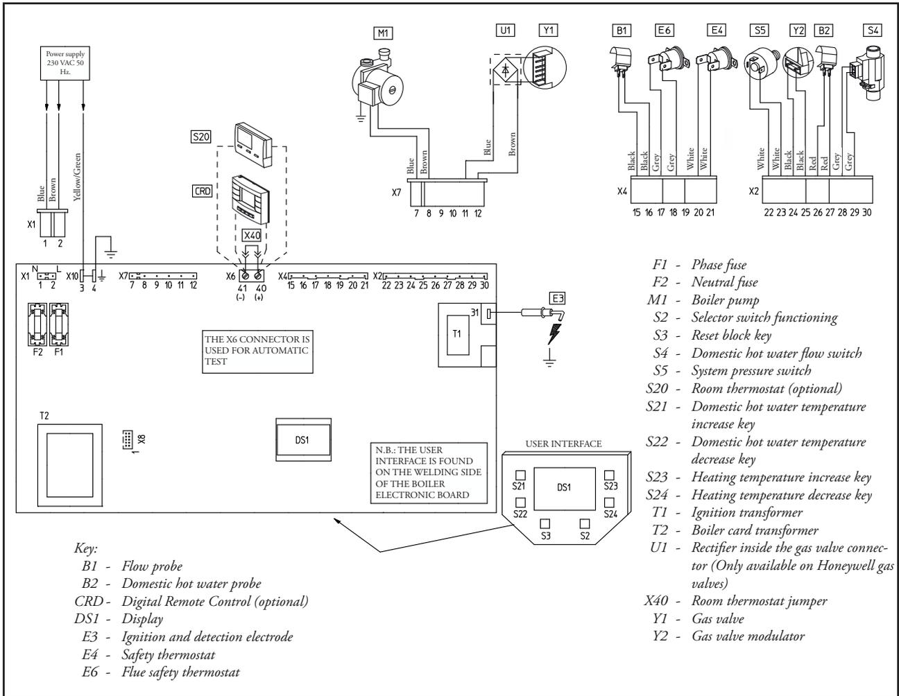
The electric circuit of the NIKE Star 24 3 E is completely interlocked to a P.C.B. with integrated microprocessor, which controls the functions of the generator. The control and safety devices partly operate at network voltage (230 V AC) and partly at low voltage.
